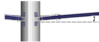
The spreader brackets are angled 6° for optimum rig support.
